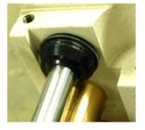
new oil seal on the needle bar bushing, shape of bushing is different
