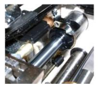
new oil seal on the looper bar bushing, shape of bushing is
